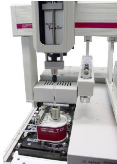
Transfer to desorption unit
