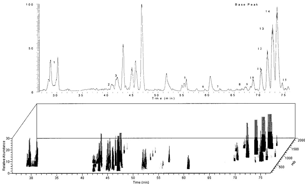
**FIG. 4.** HILIC/MS base peak chromatogram of *Cucurbita maxima* phloem, presented in a map view (TSK Gel Amide 80, gradient to 60% B was completed at 90 min). Identified peaks are (1) 3-*O*-[ $\beta$ -D-xylopyranosyl-(1-6)- $\beta$ -glucopyranosyl]-(3*R*)-octen-3-ol, (2) UDP(NAc)Gal, (3) UDPGlc, (4) DAB, (5) stachyose, (6) verbascose, (7–15) *O*-glycans.
