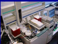
Setup of a GC/TOF instrument with automatic two-step derivatization (red ovens) and liner exchange. Both liners and vials are crimped with magnetic caps for transport.
